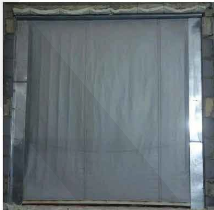
Fig. 6 Unexposed Side to Temperature/Time Resistance Test after 60 Minutes
